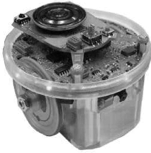
Figure 4: Miniature mobile e-puck robot.
