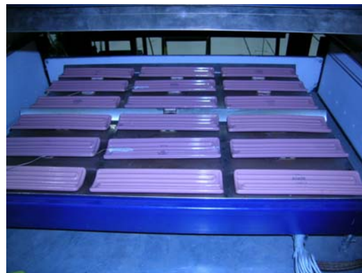
Fig. 2 (a): Heating Elements in the Bottom Tray
