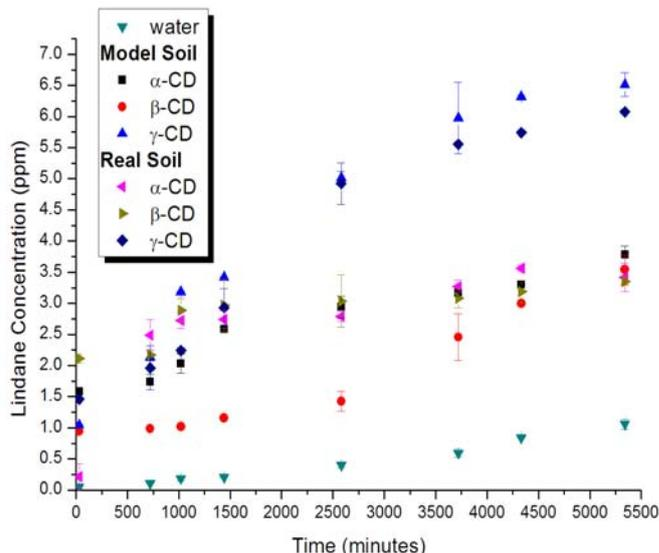
Figure 8. Lindane desorption from soils using CDs solutions and water in a *Batch* system
