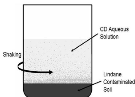
Figure 3. Batch system used along this study
