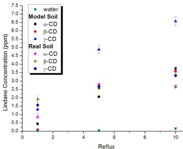
Figure 9. Lindane desorption from soils using CDs solutions and water in a column system
