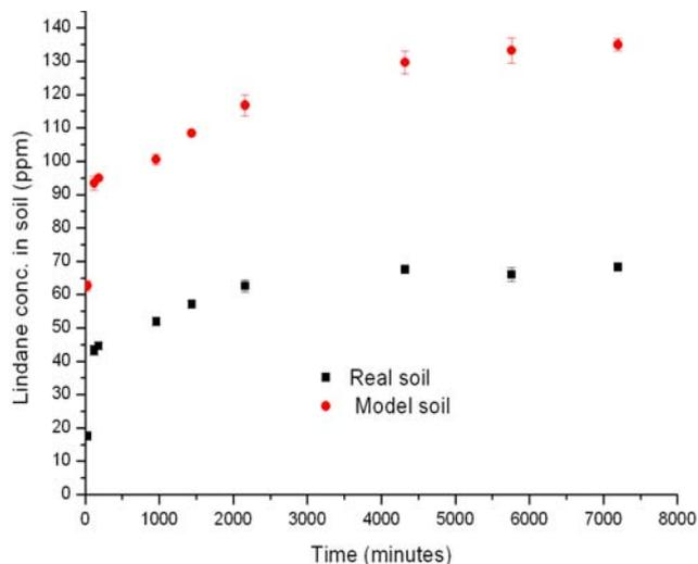
Figure 7. Lindane retention on real and model soils
