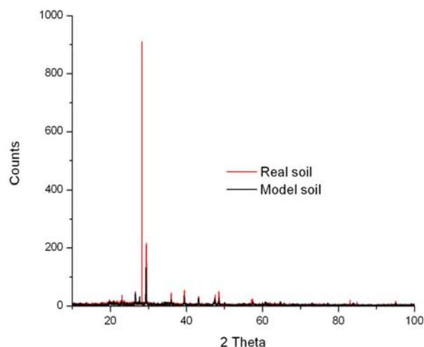
Figure 4. X-Ray diffraction of real and model soils
