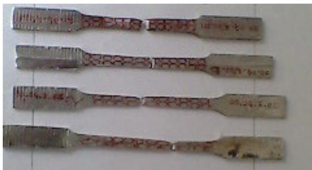
Fig. 6 : Failed Specimens
