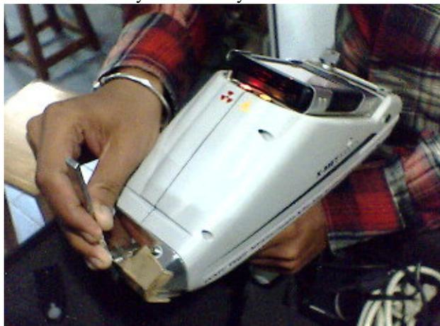
Fig. 2: Material Testing Using X-Ray Alloy Analyzer
