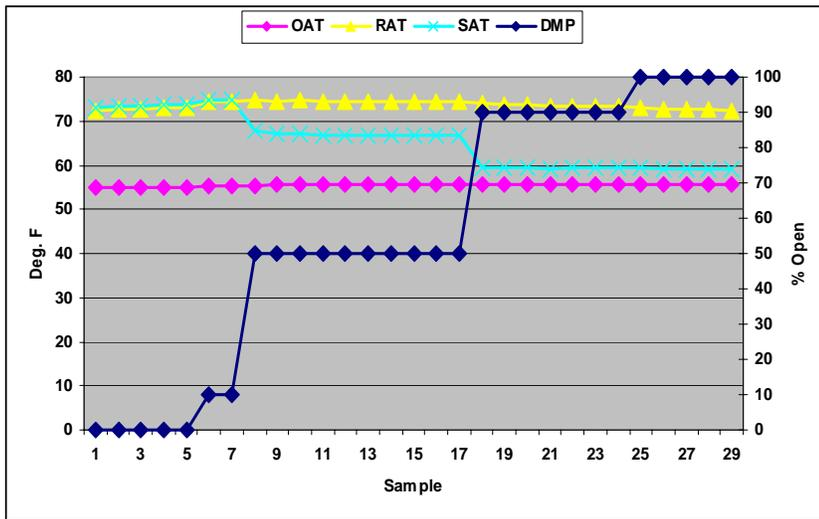
Figure 9, OAT: outside air temperature, RAT: return air temperature, SAT: supply air temperature, DMP: damper. The data is from a test run on one of the air handing units at Iowa energy center. The diagnostic result is shown in Figure 10
