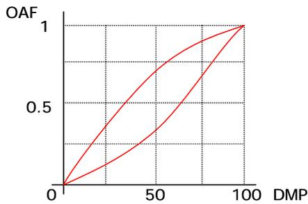
Figure 6, OAF versus damper in non-faulty mode
