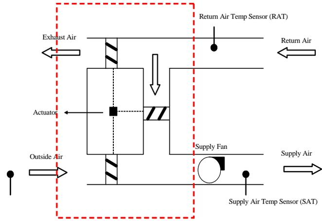
Figure 5, Schematic Diagram of Mixing Box
