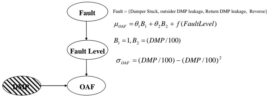
Figure 8, Fault diagnosis design for mixing box
