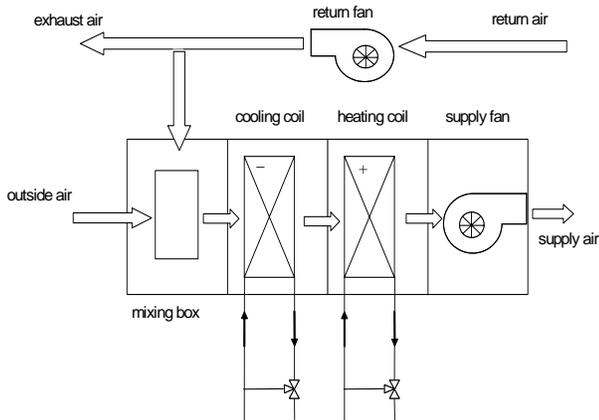
Figure 4, Schematic Diagram of Air Handling Unit
