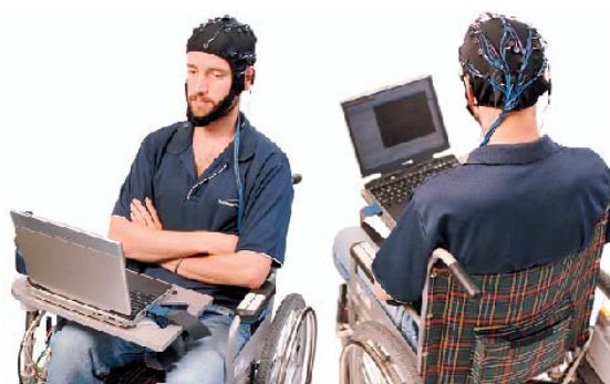
Fig. 2 A mind controlled wheelchair using EEG and a programmed computer using BCI 2000 software
