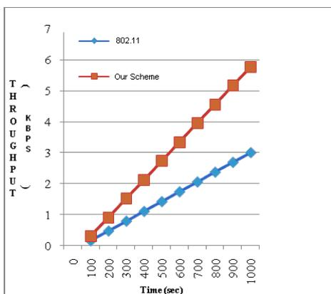
Figure 1: Throughput comparison of our scheme with 802.11
