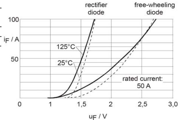
Fig. 8. Different voltage drops of rectifier and switching diodes.
