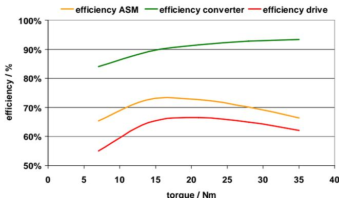
Fig. 14. Efficiency of drive components with 4 kHz pulse-frequency and varying load conditions.
