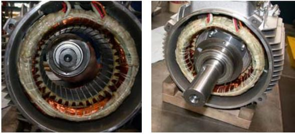
Fig. 5. A typical 5.5kW low voltage 4-pole squirrel cage induction (left) and buried permanent magnet (right) machine design.
