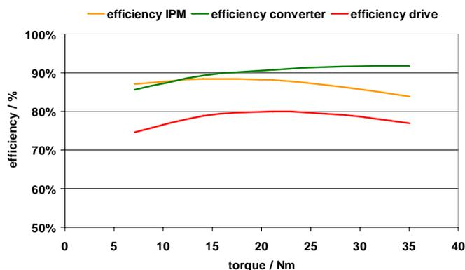
Fig. 18. Efficiency of drive components with 4 kHz pulse-frequency and varying load conditions.
