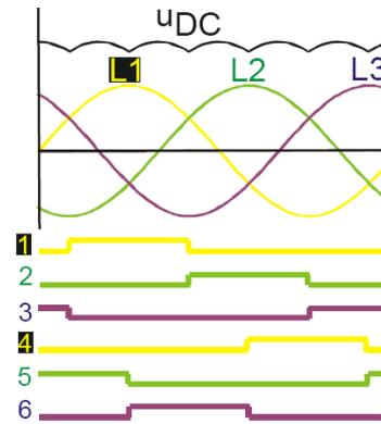
Fig. 7. Line voltage synchronizes the switching pattern for the anti-parallel IGBTs of the rectifier.
