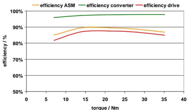
Fig. 12. Efficiency of drive components with 4 kHz pulse-frequency and varying load conditions.
