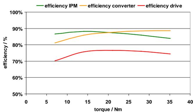
Fig. 19. Efficiency of drive components with 8 kHz pulse-frequency and varying load conditions.
