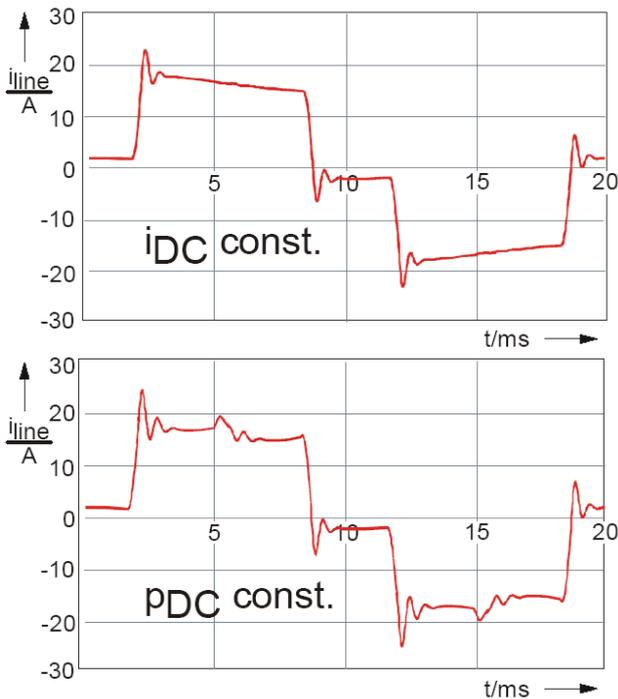
Fig. 10. Schematically line current waveforms of the fundamental frequency front end converter with line filter.
