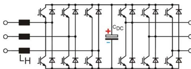
Fig. 3. Drive converter with line-side step-up inverter (active front end), DC-link and DC-AC drive inverter.
