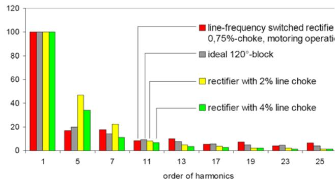
Fig. 11. Spectra of the line current for different rectifier circuits.
