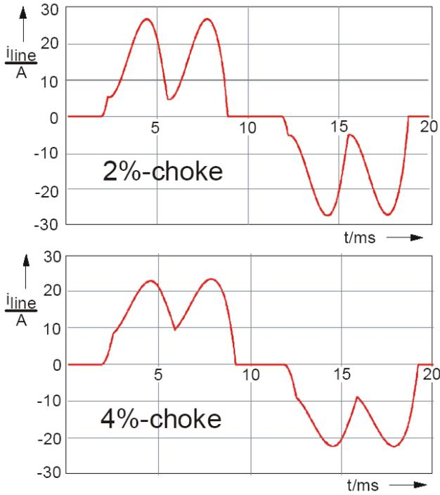
Fig. 9. Schematically line current waveforms of the standard rectifier with 2% and 4% choke.
