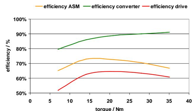
Fig. 15. Efficiency of drive components with 8 kHz pulse-frequency and varying load conditions.
