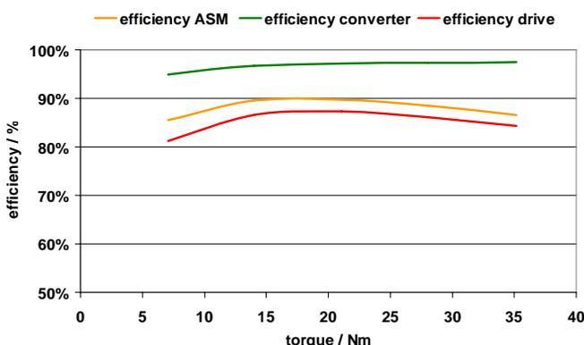
Fig. 13. Efficiency of drive components with 8 kHz pulse-frequency and varying load conditions.
