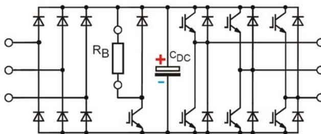
Fig. 2. AC-AC converter with AC-DC diode rectifier, DC-link capacitor with brake resistor and brake chopper as well as DC-AC drive inverter.
