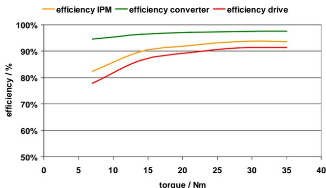
Fig. 16. Efficiency of drive components with 4 kHz pulse-frequency and varying load conditions.
