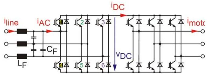
Fig. 6. Converter with line-frequency switched rectifier but without DC-link components.
