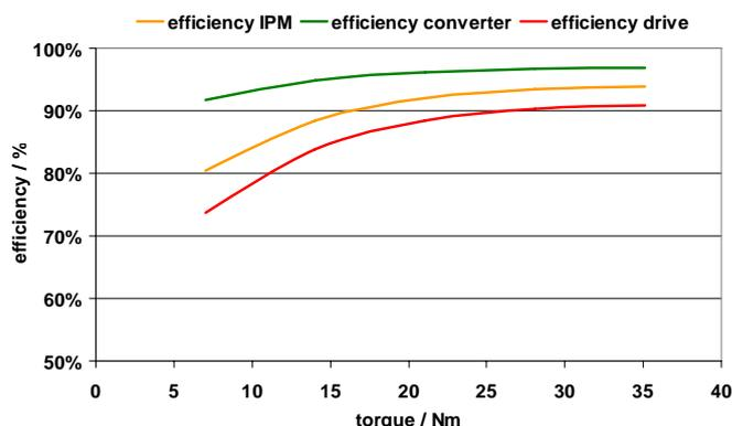
Fig. 17. Efficiency of drive components with 8 kHz pulse-frequency and varying load conditions.
