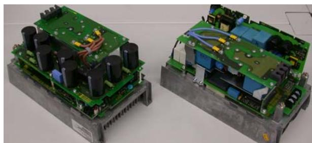
Fig. 4. State-of-the-art DC-link design (left) versus the novel line-frequency switched rectifier without DC-link (right) topology.
