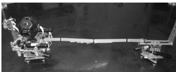
Figure 3: SPHERES with a docked flexible beam
