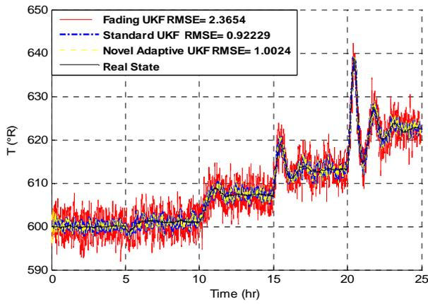
Fig.5.Estimation of Temperature of CSTR
