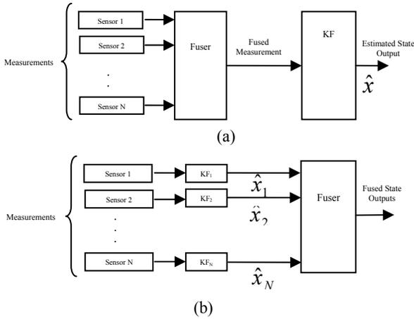
Figure 1. Kalman-filter-based multi-sensor data fusion. (a) Measurement fusion (b) state-vector fusion.
