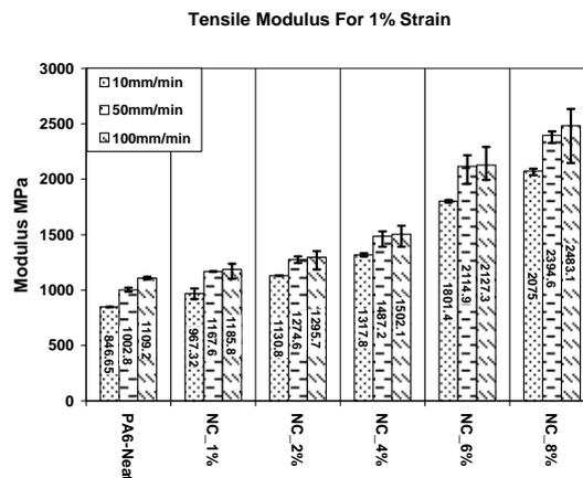
Figure 2. Column chart of elastic modulus below 1% strain
