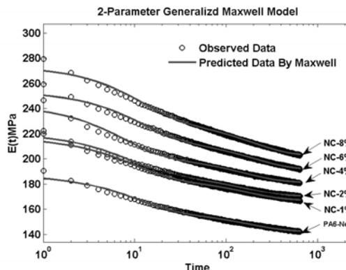
Figure 5. Stress-relaxation test results in 10% strain.
