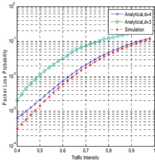
**Fig. 4. Variation of Packet Loss Probability with Traffic Intensity Over the Time-Scale [ $10^2, 10^7$ ] when  $d=3, 4$  for analytical results and when  $H=0.7$**
