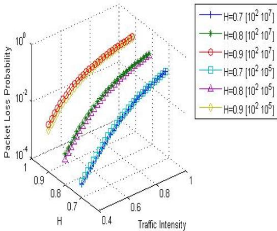
**Fig.3. Variation of Packet Loss Probability with Traffic Intensity and H when  $d = 4$ .**
