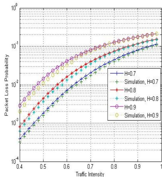
**Fig.2. Variation of Packet Loss Probability with Traffic Intensity over the Time-Scale  $[10^2, 10^7]$  when  $d=4$ .**
