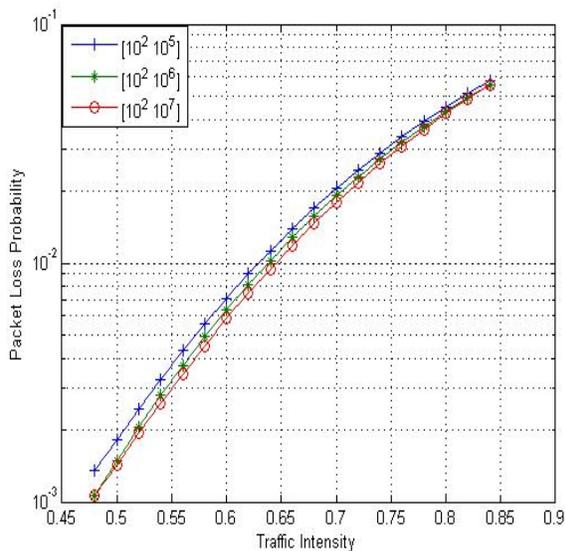
**Fig.1. Variation of Packet Loss Probability with Traffic Intensity when  $H=0.7$  and  $d=4$ .**
