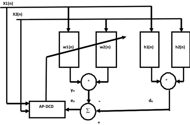
Figure 1: Block Diagram of Multichannel AP-DCD Adaptive Filtering Algorithm
