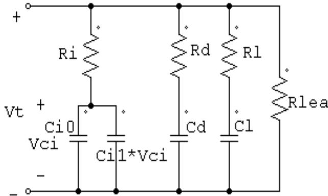
Fig.1. Equivalent Circuit Model for DLC
