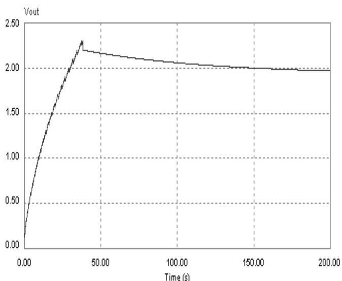
Fig.6. Simulated Output of Immediate & Delayed Branches using PSIM.
