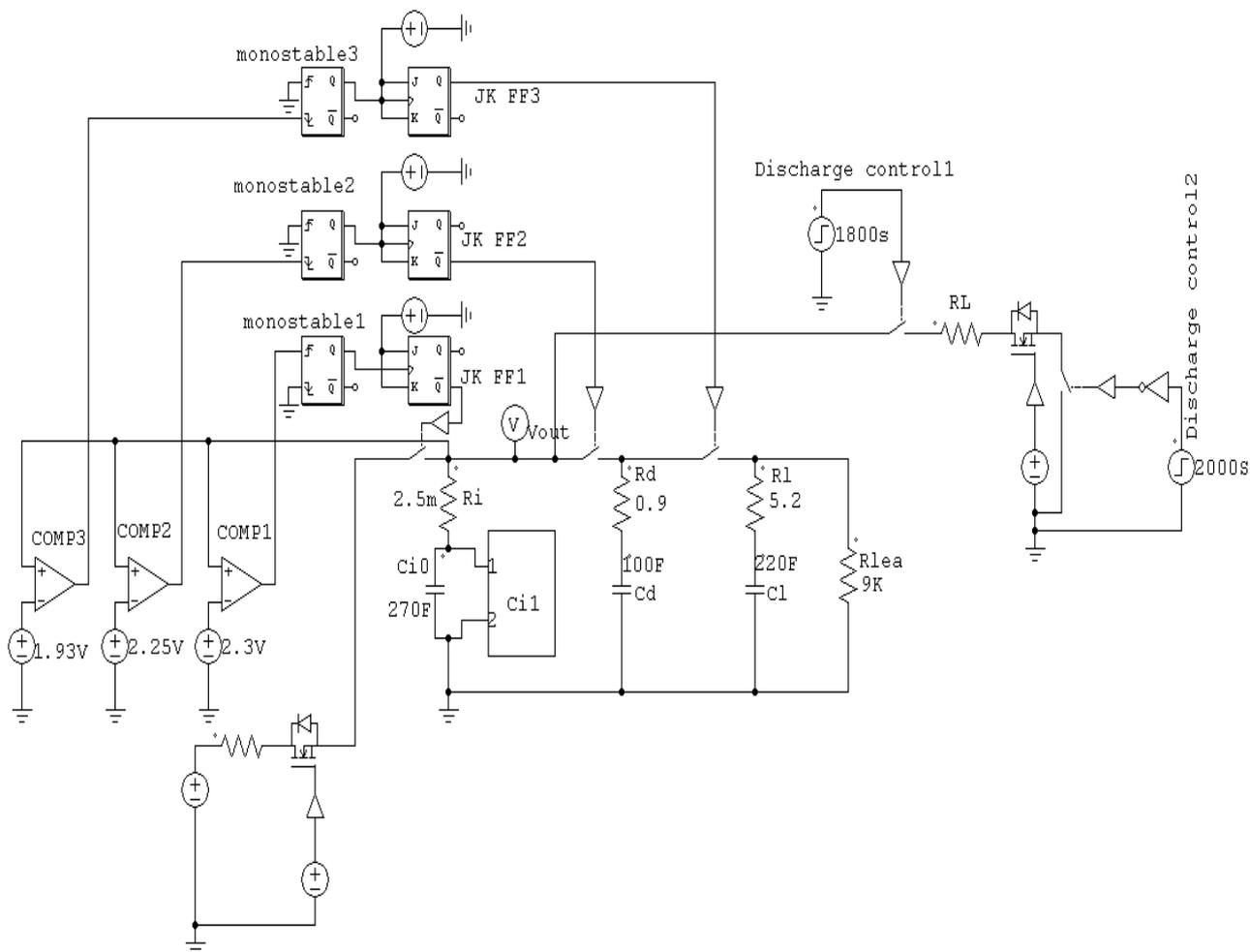
Fig. 3. Equivalent Circuit Model of a DLC with Charge-Discharge Control Circuitry.
