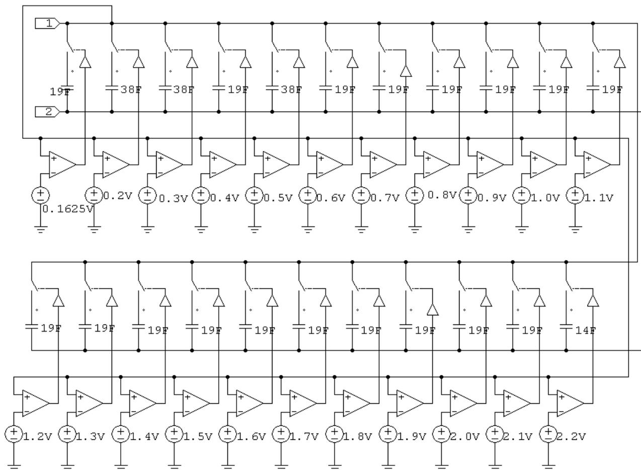
Fig.2. Voltage Dependent Capacitor Simulated using PSIM
