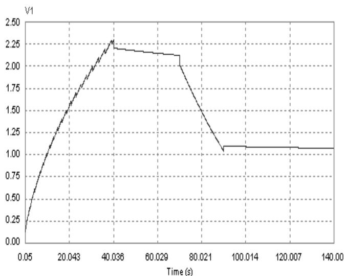
Fig.7. Simulated Output of EDLC Model using PSIM.
