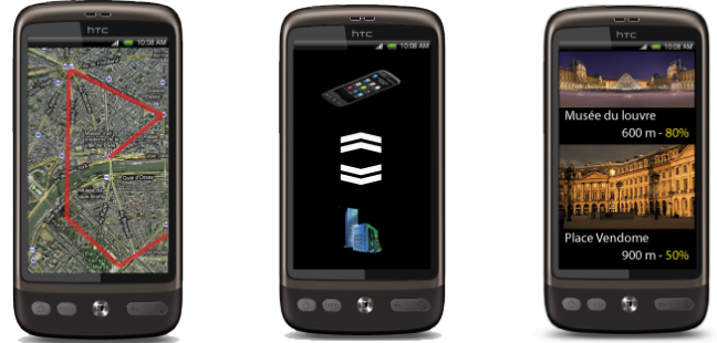
Fig. 6. Main steps of the mobile application: (a) Along the user visits, application build the gps trace. (b) the trace is sent to the server that computes distance to select sites. (c) Results are shown to the user.
