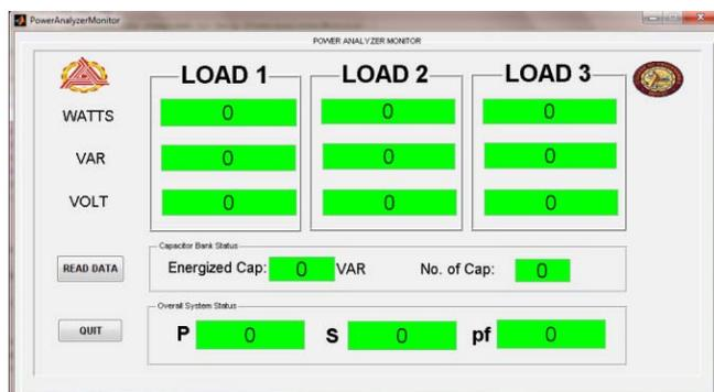
**Fig. 6** Power Monitoring Software
