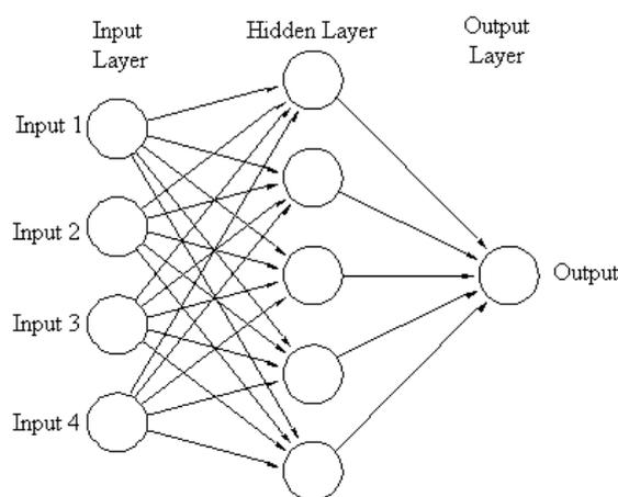
Fig. 1 Artificial Neural Network Diagram
