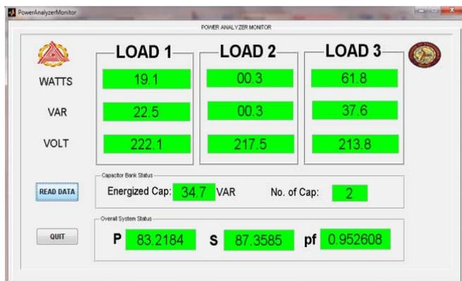
**Fig. 8** Sample of Working Controller with Two (2) Capacitors Energized
