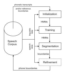
Fig. 2. Scheme of automatic acoustic inventory creation.
