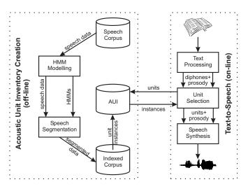
Fig. 1. Block diagram of ARTIC TTS system.
