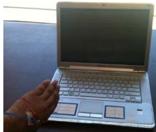
Fig. 4. Hand motion test with wearable accelerometer tilted right and facing up
