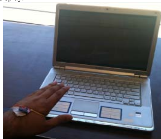
Fig. 6. Hand motion test with wearable accelerometer straight up
