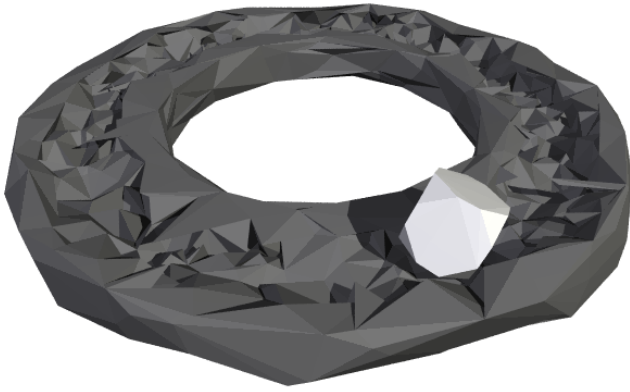
Fig. 6. Simulated Machined Workpiece and Diamond Grain.
