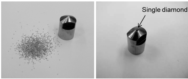
Fig. 1. Sample Before and After Brazing.
