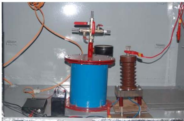
Figure 1. Photograph of the high pressure test chamber
