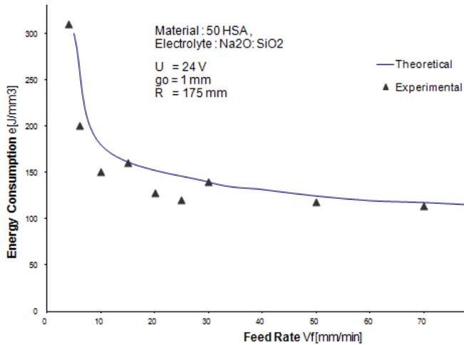
Figure 7. Specific energy consumption vs. feed rate
