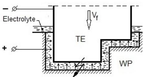
Figure 1. Scheme of ECDM/ECAM
