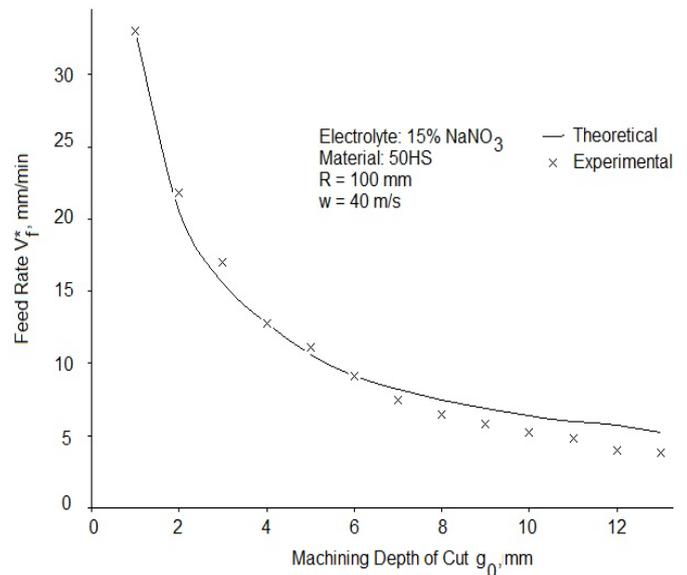
Figure 6. Critical feed rate vs. depth of machining
