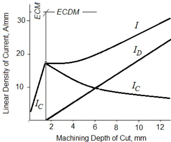
Figure 4. Effects of machining depth of cut and feed rate on linear current density
