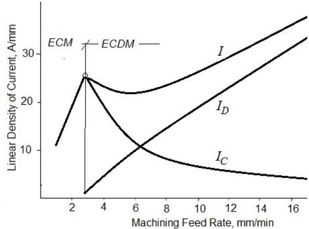
Figure 5 Effects of machining feed rate on linear current density
