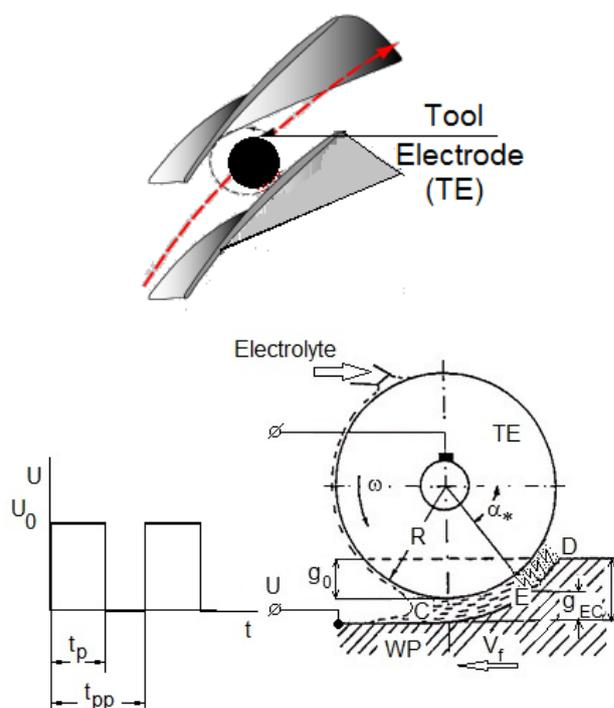
Figure 2. Schematic diagram of Rotary Electrochemical Discharge Machining
