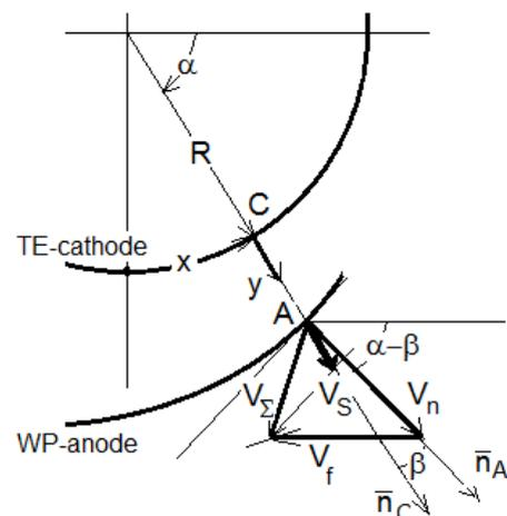
Figure 3. Scheme for modeling of electrochemical shaping
