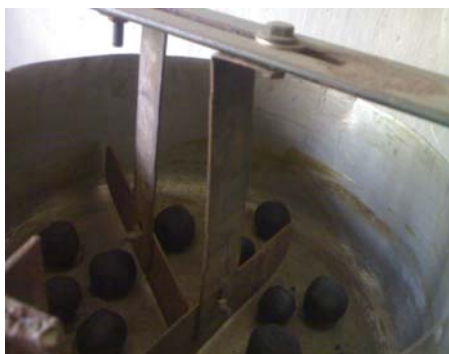
Fig 6: Plane view of the balling disc machine
