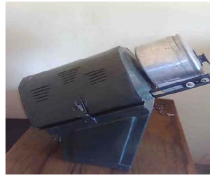
Fig 3: The side view of the balling disc machine
