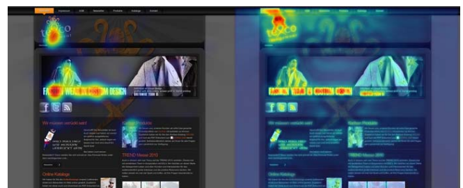
Fig. 1. Eye-tracking output (left) and automated attention analysis [13] Captured snapshots of a website are analyzed on various features such as color, orientation, density, contrast, intensity, size, weight, intersection, closure, length, width and curve of displayed objects. Text, skin color and face detection are also included [14]. Other tools may identify as many as 50 other features which attract human attention the most [15].
