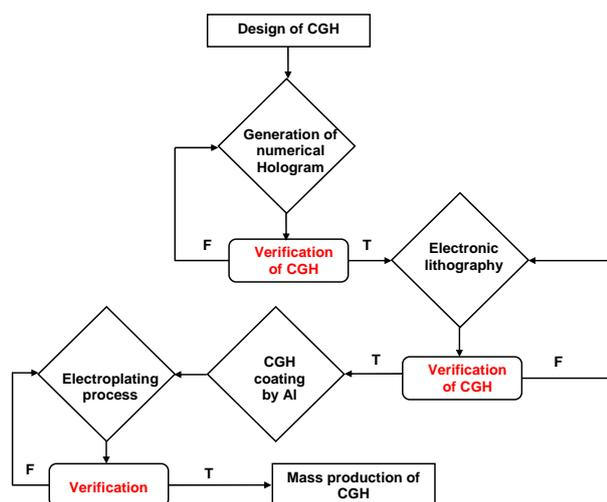
Fig. 1. Algorithm for manufacturing of microstructure: from design of CGH to mass production
