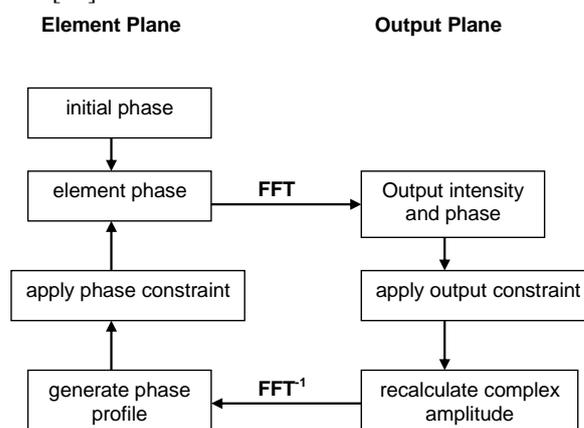
Fig. 2. A schematic representation of the Gerchberg-Saxton algorithm.
