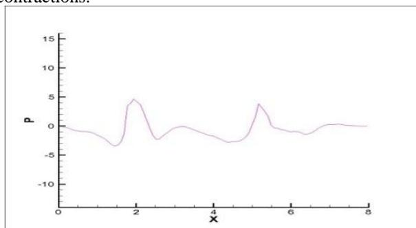
Fig 4. Instantaneous pressure distribution (dyn/cm<sup>2</sup>) along the centre line(cm).
