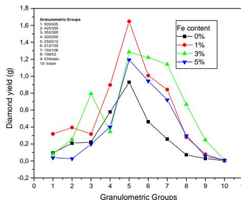
Figure 2 - Correlation between the diamond productivity and the granulometry of synthesized crystals for the different Fe contents.
