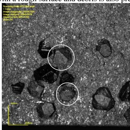
Figure 4 – Confocal micrograph of worn surface of a segment produced with commercial diamonds
