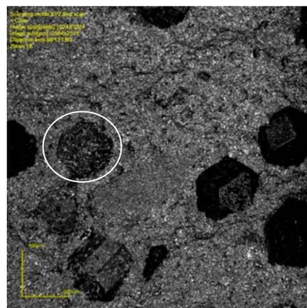
Figure 5 – Confocal micrograph of worn surface of a segment produced with diamonds obtained in this research
