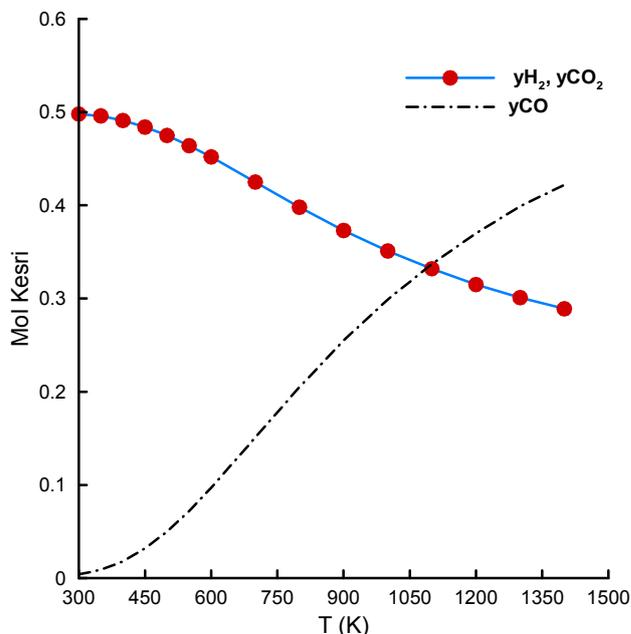
Fig. 4. Equilibrium compositions of gaseous mixture versus reaction temperature on water free basis (1 mol CO+1 mol H<sub>2</sub>O)
