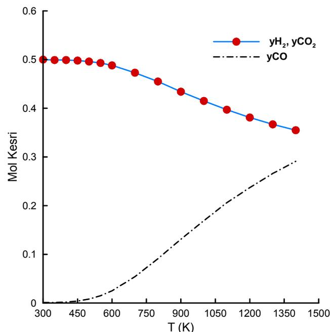
Fig. 5. Equilibrium compositions of gaseous mixture versus reaction temperature on water free basis (1 mol CO+2 mol H<sub>2</sub>O)
