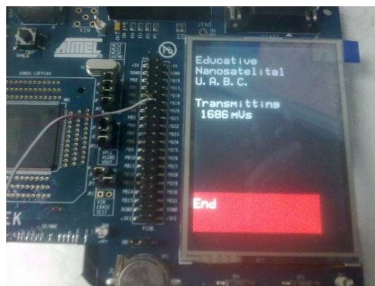
Fig. 9. Displaying measured voltage on touch screen
