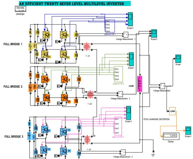
Fig. 7. Simulation diagram for an Efficient 27- Level Multilevel Inverter with L-Load
