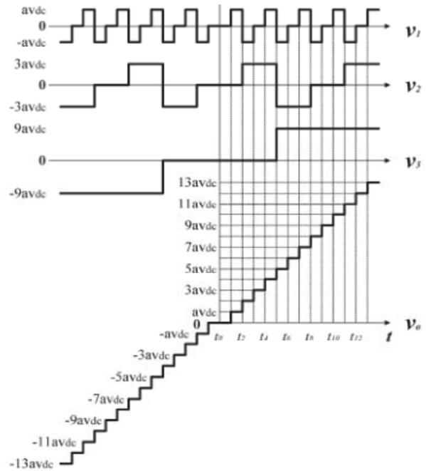
Fig. 4. Expected output voltage levels and each terminal voltage of the transformer
