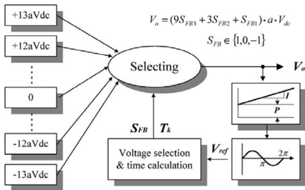
Fig. 6. Control block diagram of the proposed multilevel inverter
