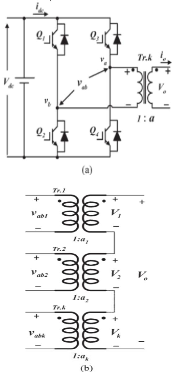
Fig. 2. Basic concept of the proposed multilevel waveform synthesis; (a) Single phase full bridge inverter module; (b) Cascaded connection of the secondary winding of the transformer
