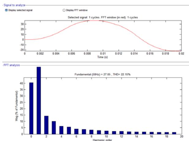
Fig. 11. FFT Analysis for Resistive load
