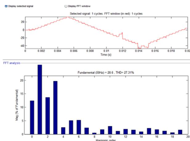
Fig. 12. FFT Analysis for Inductive load
