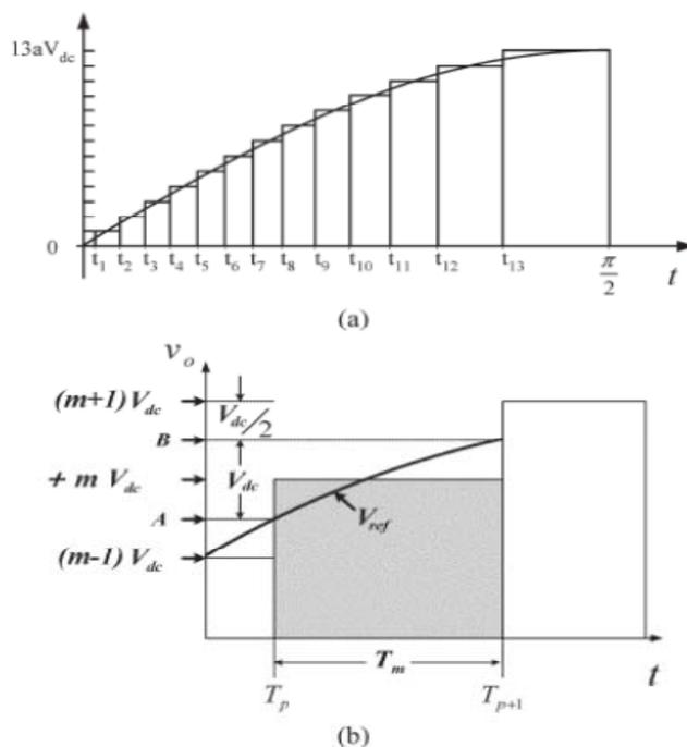
Fig. 5. Reference and output voltage of the proposed multilevel inverter a) Reference and output voltages for ¼ cycles; b)Determination of corresponding duration
