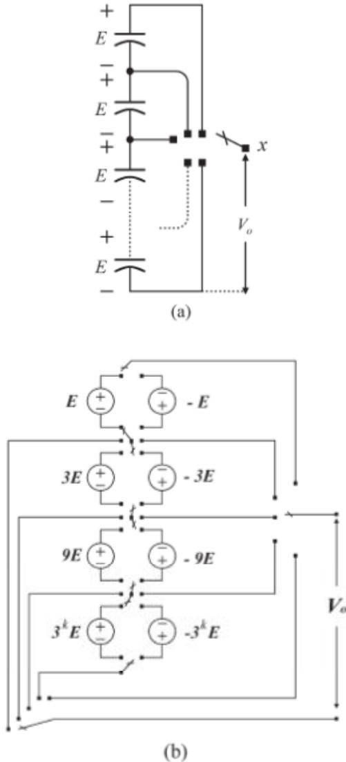
Fig. 1. Basic concept of the general and proposed multilevel waveform synthesis a) General approach; b) proposed method
