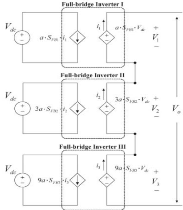
Fig. 3. Equivalent circuit of the proposed multilevel inverter employing cascaded three transformers with a series connected secondary winding
