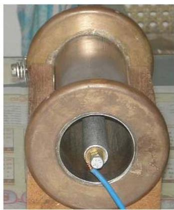
Figure2. Photograph of the Co-axial Duct
