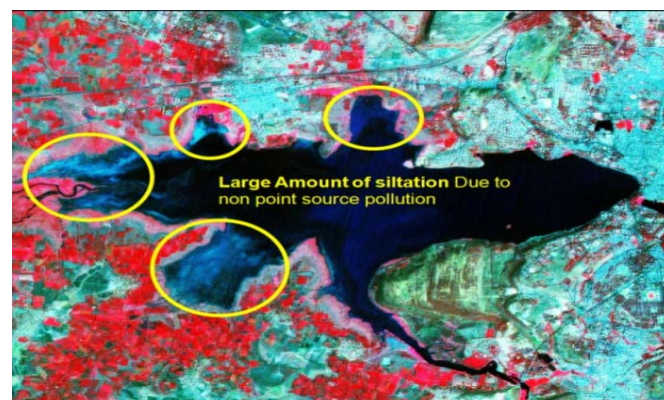
Fig 15- Siltation in Lake catchment area.
