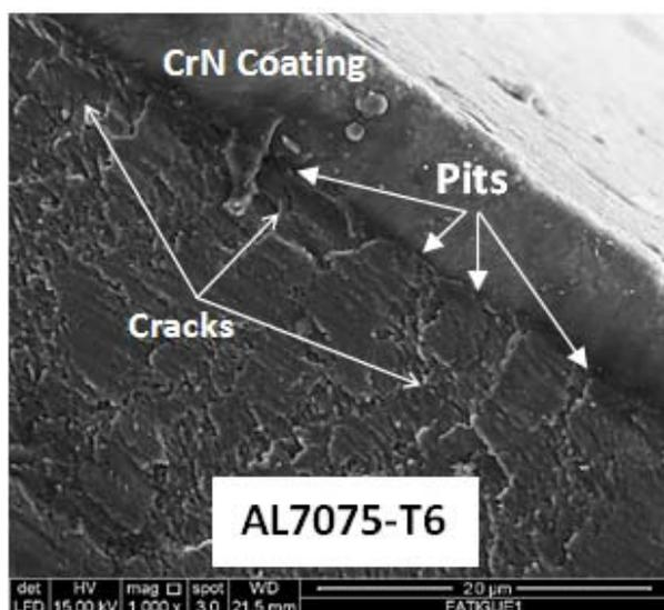
Fig. 8 Typically SEM micrograph of CrN coated specimen with adhesion of 2200 (mN) after fracture at stress of 200 MPa.
