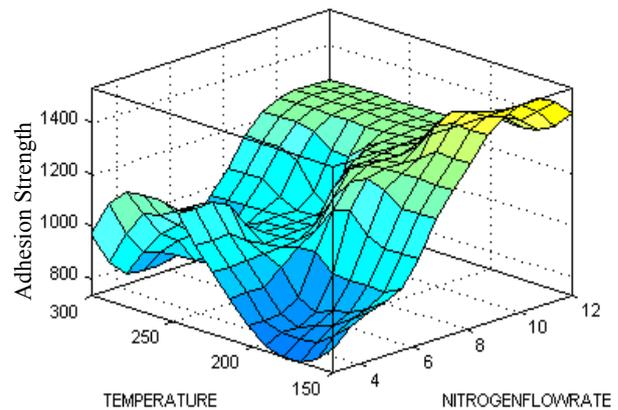
(a) Adhesion strength in relation to change nitrogen flow rate (C) and
