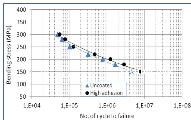
b) S/N curve of fretting fatigue for uncoated and Cr-CrN coated with highest surface adhesion specimens
