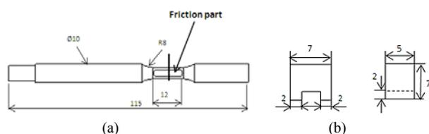
Fig. 1 Drawings of the fretting fatigue specimen and the fretting pad
