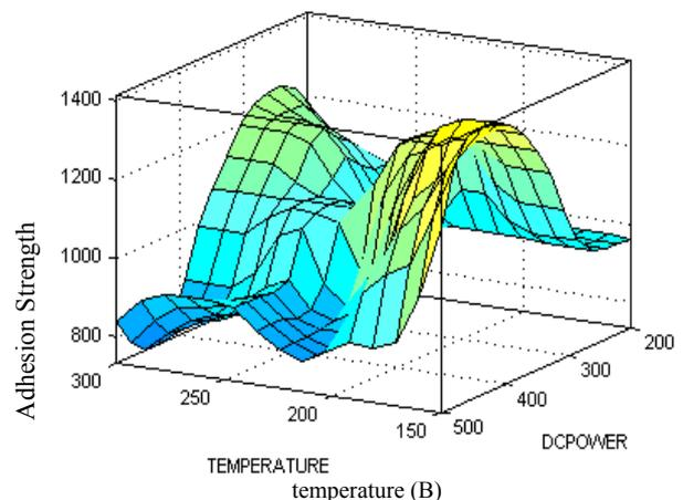
(b) Adhesion strength in relation to change DC power (A) and temperature (B)
