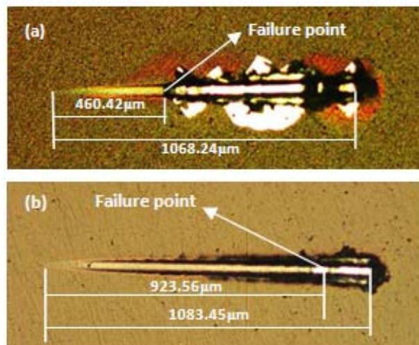
Fig. 3 Adhesion strength of Cr-CrN coated samples at different condition (a) weak adhesion (DC power 500W, temperature 150 and nitrogen flow rate 3%, scratch force 510 mN) and (b) strongest adhesion (DC power 300W, temperature 250 and nitrogen flow rate 9%, scratch force 2200 mN)
