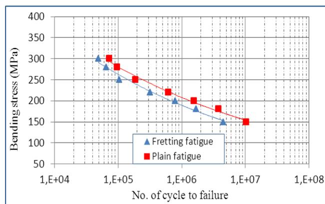
(a) S/N curve of plain fatigue and fretting fatigue for uncoated specimens
