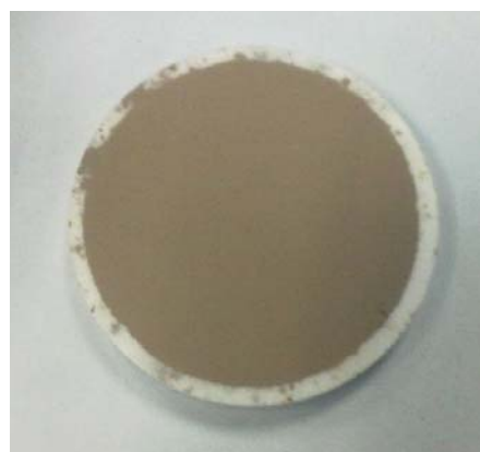
Fig. 4 Tablet produced for XRF analysis
