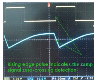
Fig 8. Zero-crossing detector Signal and Ramp Signal from Integrator Output
