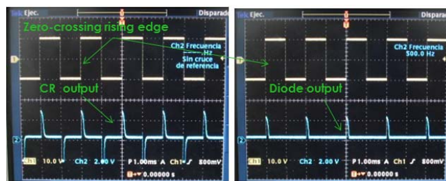
Fig 9. CR output and final diode output (energy signal centre)
