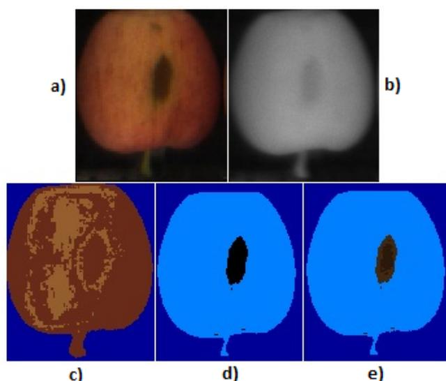
Fig. 2: Example of a Gala apple with a blemish, imaged under the (a) visible and (b) infra-red spectra. Example of the manual process of selecting dominant fruit colours and that of the conveyor belt in order to achieve segmentation (c). Identification of the blemish region within the segmented image (d) and the manual identification of the dominant colours representing the blemish region (e).
