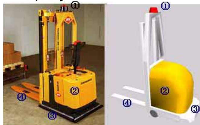
Fig.2 The comparison of the real AGV and the simulation model
