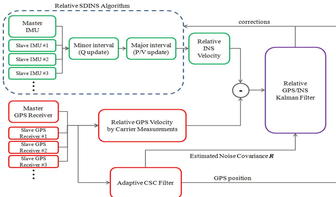
Fig. 1. Architecture of proposed adaptive GPS/INS algorithm.
