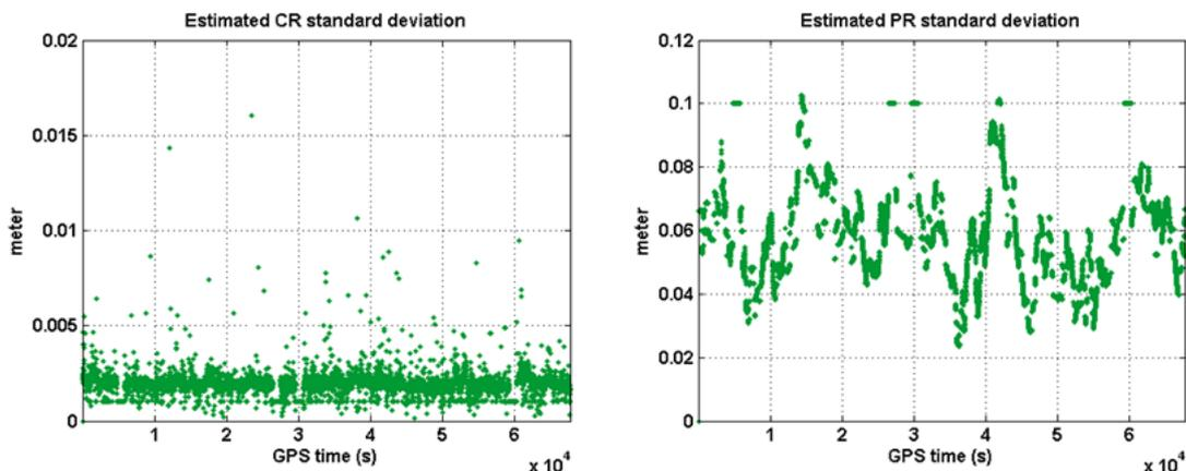
Fig. 2. Estimated standard deviations for carrier-phase and pseudorange noise terms.
