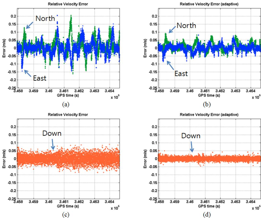
Fig. 3. Comparison of relative velocity errors in north, east and down directions
