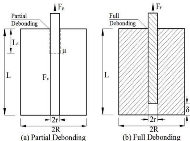
Fig. 2 Interfacial debonding between single fiber and resin matrix
