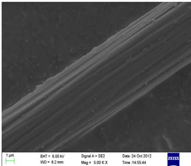
Fig. 4 Surface morphology of carbon fiber with combined treatment × 5000
