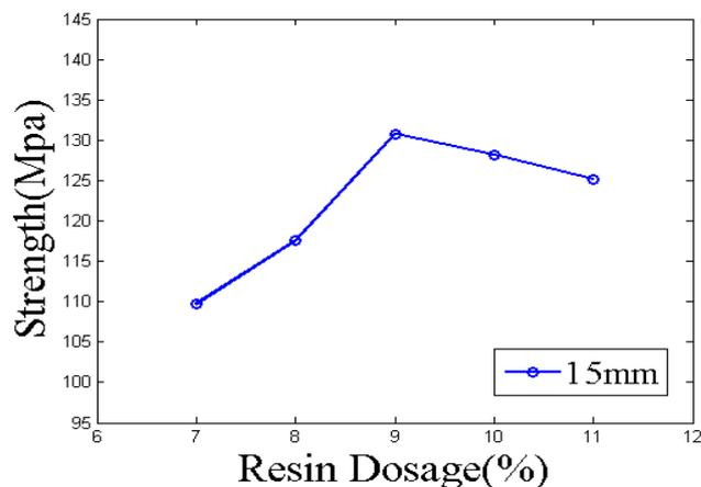
Fig.6 Relationship between strength and resin dosage
