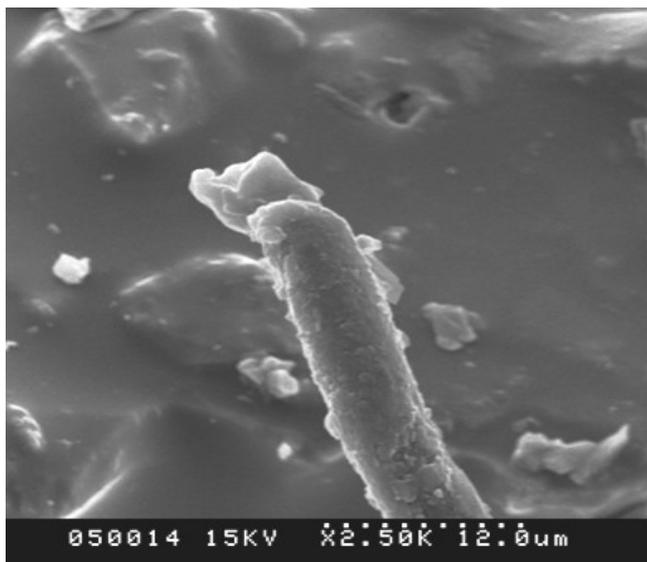
Fig. 7 Surface attachment of carbon fiber
