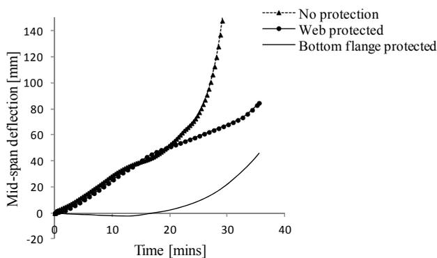
Fig. 13 Mid-span deflection for test beam 1 for different protection schemes
