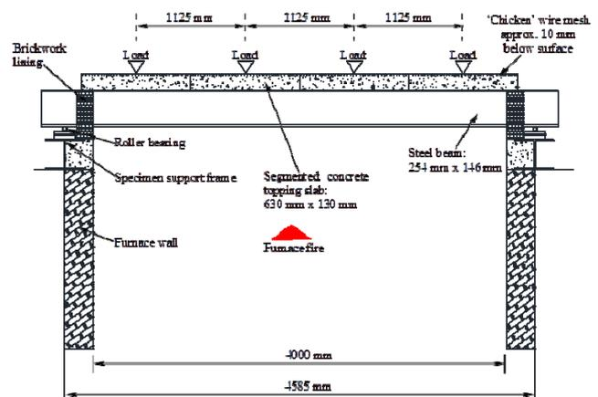
Fig. 6 Longitudinal section for the simply supported floor beam test 2 assembly [16]
