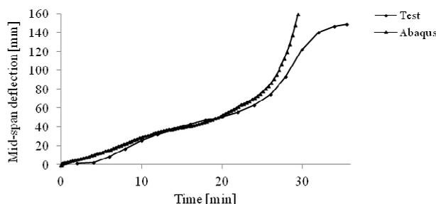
Fig. 9 Mid-span deflection for test beam 1
