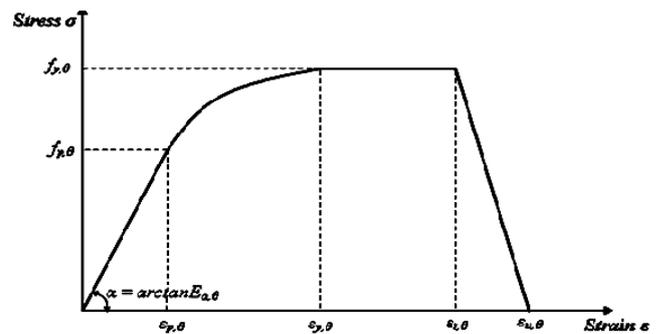
Fig. 3 Stress-strain model for carbon steel
