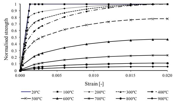
Fig. 4 Stress-strain-temperature curves for carbon steel
