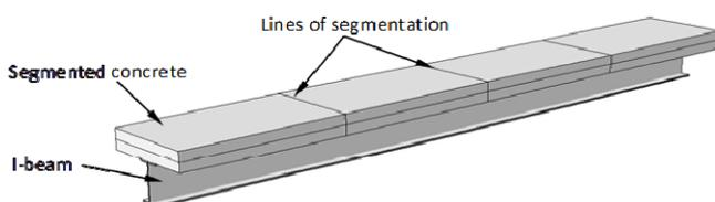
Fig. 5 The beam model carrying segmented floor slabs
