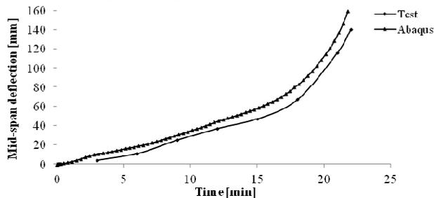
Fig. 11 Mid-span deflection for test beam 3
