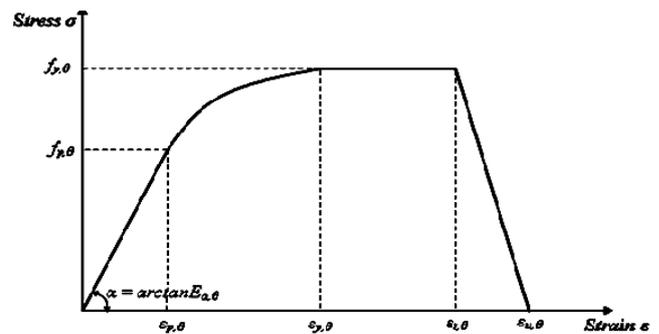
Fig. 3 Stress-strain model for carbon steel
