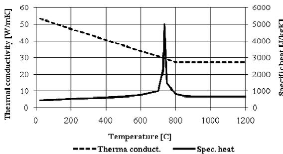
Fig. 1 High temperature thermal properties of carbon steel
