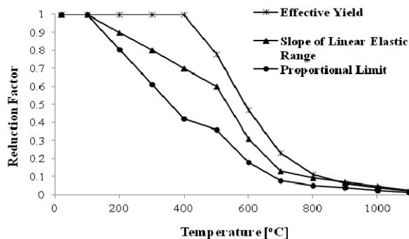
Fig. 2 Mechanical properties reduction factors for carbon steel at elevated temperatures
