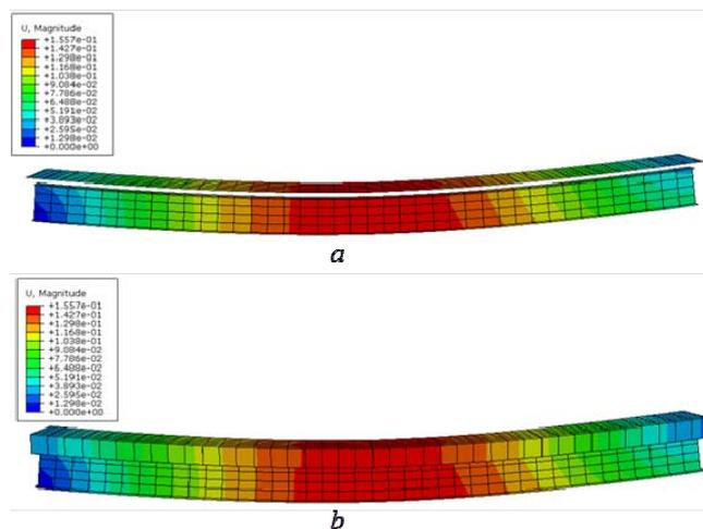
Fig. 8 Deflection profile for the numerical calculation of test beam 1 (a) Shell element (b) Rendered shell element thickness
