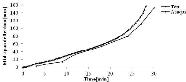
Fig. 12 Mid-span deflection for test beam 4
