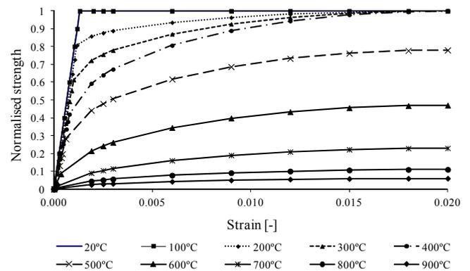
Fig. 4 Stress-strain-temperature curves for carbon steel
