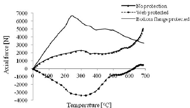
Fig. 14 Axial force in test beam 1 for different protection schemes
