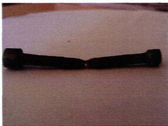
Figure 9: Fracture specimen showing a cone and cup fracture mode
