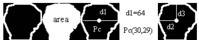
Fig. 5. The process of geometric feature extraction
