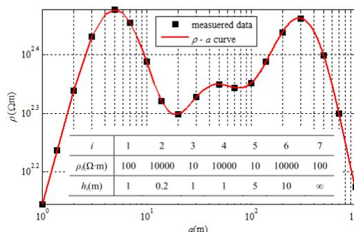
Fig.3. The  $\rho-a$  curve and measured resistivities of Wenner method using the proposed probe spacing configuration.
