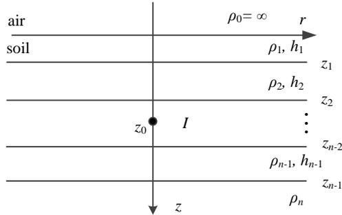
Fig.1. horizontal  $n$ -layer soil.  $\rho_j$  and  $h_j$  is resistivity and thickness of layer  $j$ .  $z_j$  is  $z$ -axis coordinate of boundary of layer  $j$  and layer  $j+1, j=1,2,\dots,n-1$ .
