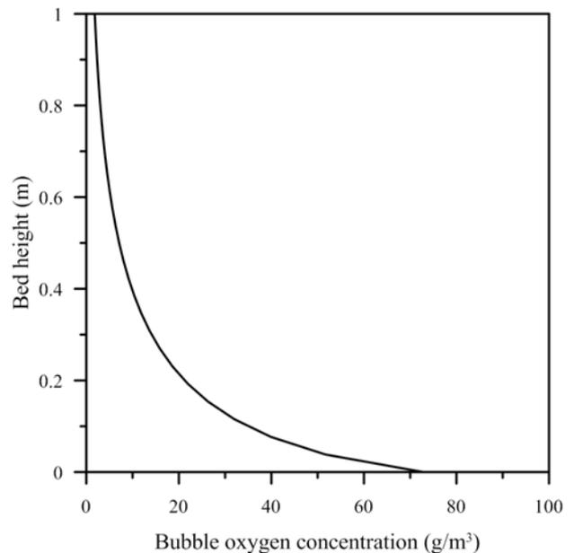
Fig. 5. Oxygen concentration profile ( $D_{bed}=1m$ ).
