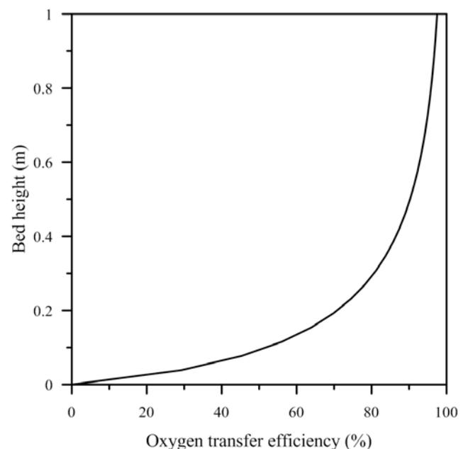
Fig. 6. Transfer oxygen efficiency ( $D_{bed}=1m$ ).
