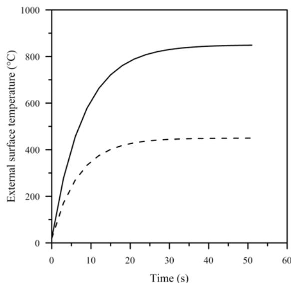
Fig. 2 Temperature increasing of the external surface of a PE pellet in a BFB at 850°C (continuous line) and 450°C (dot line).
