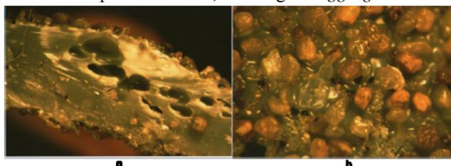
Fig. 3 Photos of a PE pellet kept 15s in BFB at 450°C. Transversal section (a); external surface (b).
