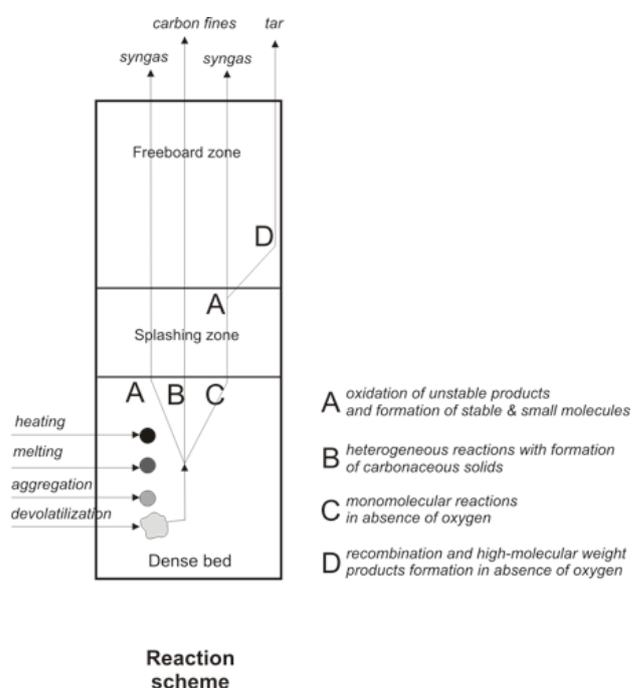
Fig. 4. Scheme of reactions as occurring in a BFB gasifier fed by plastics.
