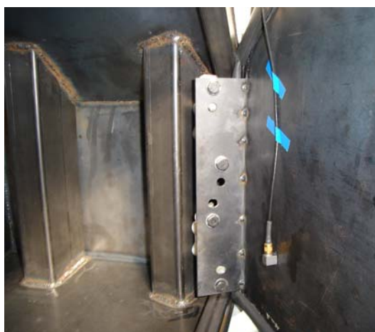
Fig. 2. Attached accelerometer at door reference point.
