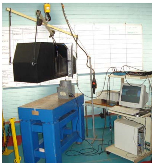
Fig. 4. Vehicle test set-up with attached microphone at driver's head location.
