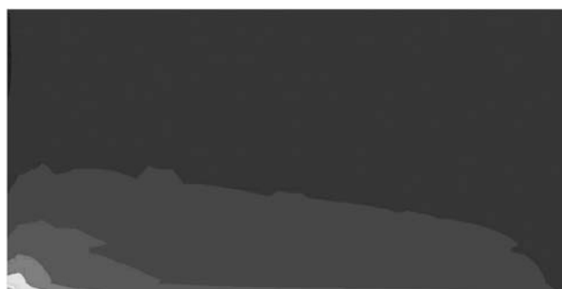
Fig. 8. Stress S1 in masonry wall strengthened with grid pattern by using CFRP strips for horizontal uniformly distributed load 200 kN/m 2 .
