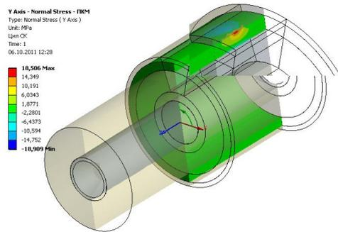
Fig. 5. Fields normal stresses  $\sigma_y$  in layer PC of layer system of type "metal - polymer composite - metal" when turning
