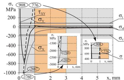
Fig. 8. Stress distribution along depth of work part in zone of load application
