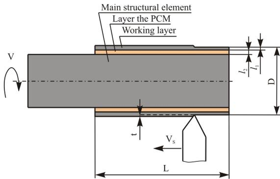
Fig. 4. Construction of layer system of type
