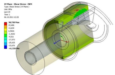
Fig. 6. Fields shear stresses  $\sigma_{XY}$  in layer PC of layer system of type "metal - polymer composite - metal" when turning
