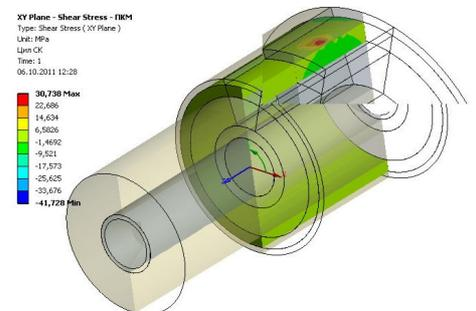
Fig. 6. Fields shear stresses  $\sigma_{XY}$  in layer PC of layer system of type "metal - polymer composite - metal" when turning
