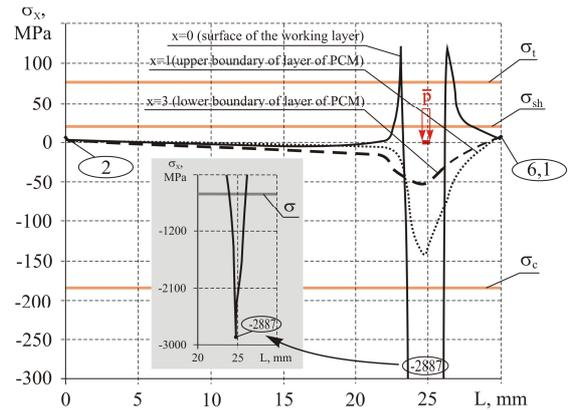
Fig. 7. Stress distribution along axis of layer system of type "metal - polymer composite - metal" when turning:  $\sigma$  - ultimate strength;  $\sigma_t$  - ultimate tensile strength;  $\sigma_{sh}$  - ultimate shear strength;  $\sigma_c$  - ultimate compressive strength
