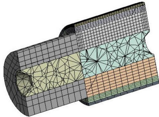
Fig. 2. Solid model of layer system while axial turning with table of finite elements
