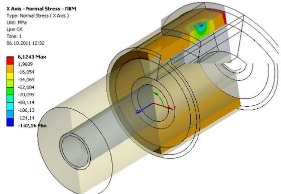
Fig. 3. Fields normal stresses  $\sigma_x$  in layer PC of layer system of type "metal – polymer composite – metal" when turning
