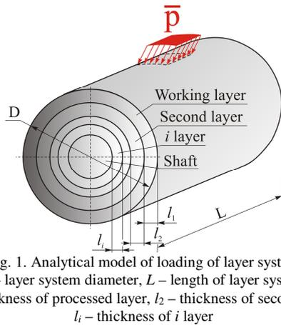
Fig. 1. Analytical model of loading of layer system
