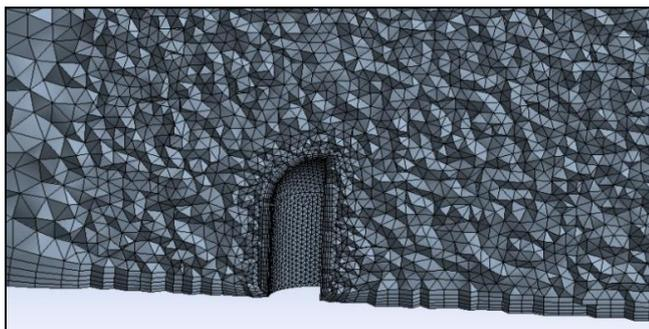
Fig.4: Close-up mesh cross section
