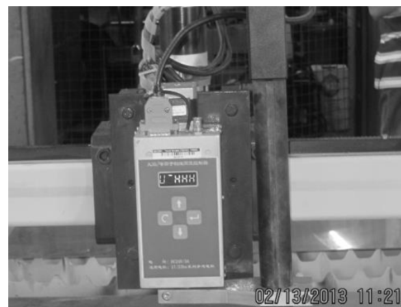
Fig. 10. Torch height controller (THC) process
