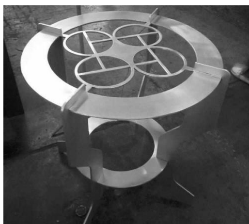
Fig. 13. Coffee table – a sample plasma cut in stainless steel diagram
