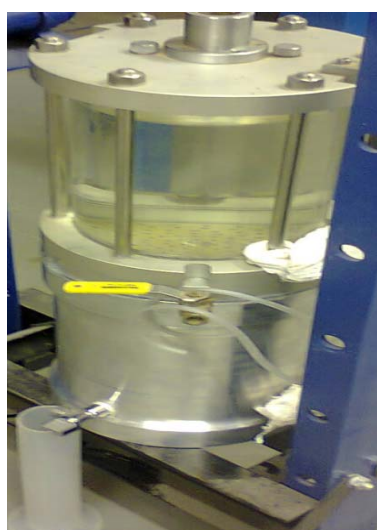
Fig. 7. Percolation test under study using de-ionized water as permeant for CCA-treated wood with the effluent collected and tested at intervals to track the concentration levels of the targeted chemical ions of concern
