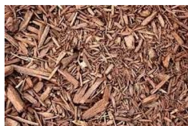
Fig. 4. CCA-treated wood chopped into smaller pieces for percolation tests
