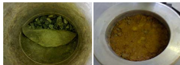
(a) Filter bed (b) Soil over CCA-treated wood Fig. 5. (a) and (b) Wet geotextile placed over selected gravel and lightly compacted clayey soil over chopped CCA-treated wood in the bucket section
