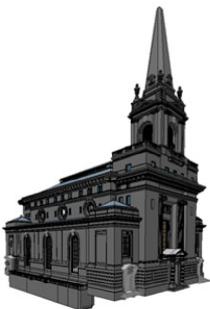
Fig. 4. Digital model of the façade of the historical church (performed by True Point LLC, http://truepointscanning.com )
